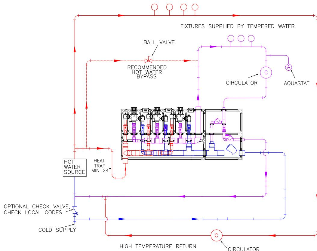
**CAUTION!** All thermostatic water mixing valves have limitations. They will NOT provide the desired accuracy outside of their flow capacity range. Consult the Flow Capacity Chart and DO NOT OVERSIZE. Minimum flow must be no less than as indicated.
