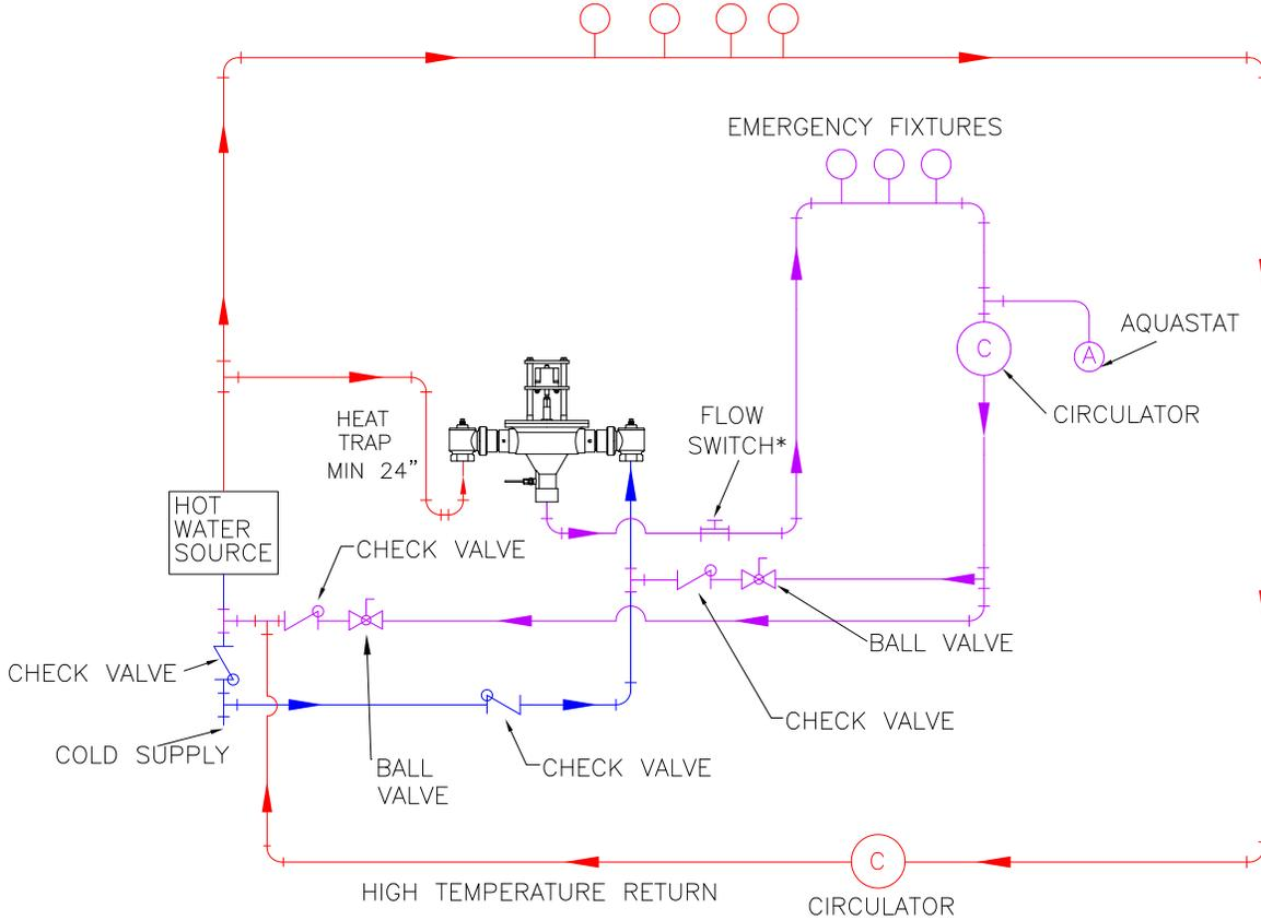
\* FLOW SWITCH MUST BE LEVEL AND IN CORRECT DIRECTION, FLOW SWITCH SHIPS INSTALLED IN TEE, COPPER TUBING TOTALLING ROUGHLY 18" INCLUDED
