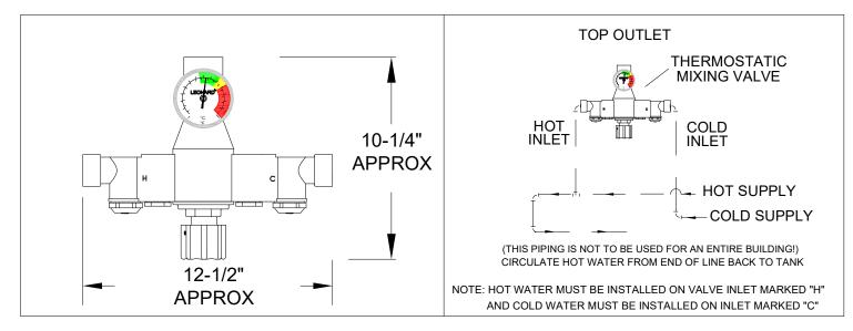
CAUTION! It may be necessary to recirculate the tempered water to the drench / eye/face wash should the piping be exposed to excessive hot or cold conditions. Consult factory for proper piping.
