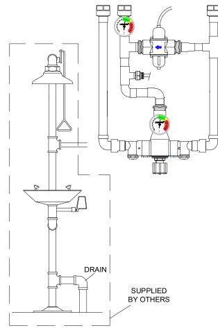
Primary Mixing Valve is certified to meet Low-Lead requirements of wetted surface area containing less than 0.25% lead by weight. All other fittings and components, the sum total of which comprise the wetted surface of this product, contain less than one quarter of one percent of lead by weight.
