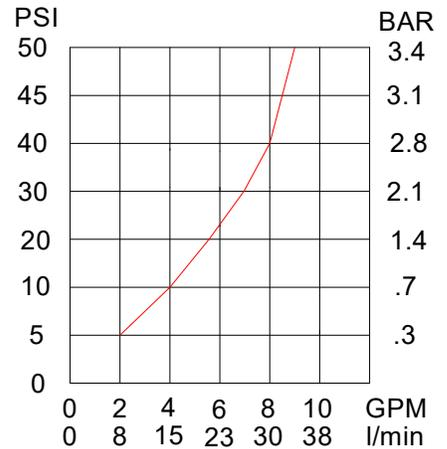
**CAUTION!** All thermostatic water mixing valves have limitations. They will NOT provide the desired accuracy outside of their flow capacity range. Consult the Flow Capacity Chart and DO NOT OVERSIZE. Minimum flow must be no less than as indicated.
